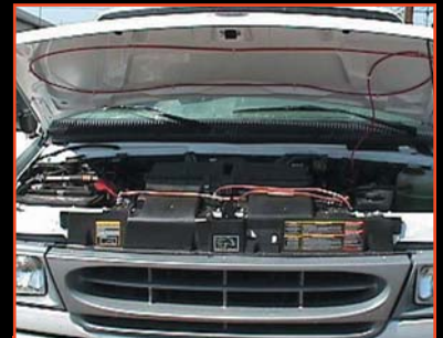
The red Firetrace Detection Tubing (pictured above and below) can be run across all potential hazard areas, ensuring detection is close to the most probable fire sources.
